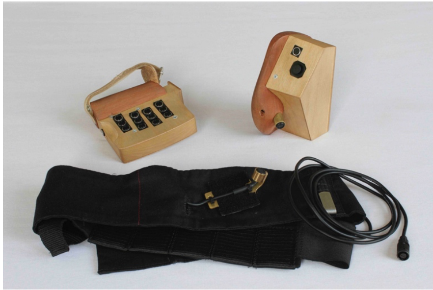
Original version of the strophonion's controller system: 1.) right hand controller (top left) displaying twelve buttons representing all twelve tones of an octave 2.) left hand controller (top right) displaying a shift button to switch functionality, 2D-joy-stick and the receiver of the ultrasonic distance sensor 3.) hip belt with the transmitter of ultrasonic distance sensor (on the bottom). © photo Janina Janke, 2014.
