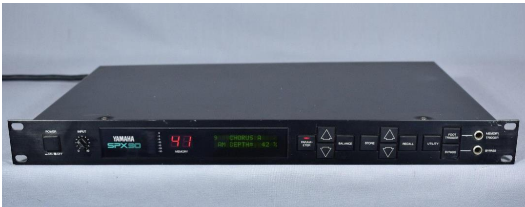
Figure 8. The Yamaha SPX90 digital multi-effects processor used by Saariaho in her earlier works with live electronics.
