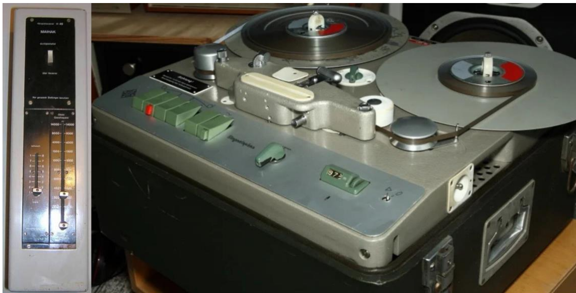
Figure 11. Maihak W 49 band-pass filter (left) and Telefunken M 5 tape recorder (right).
