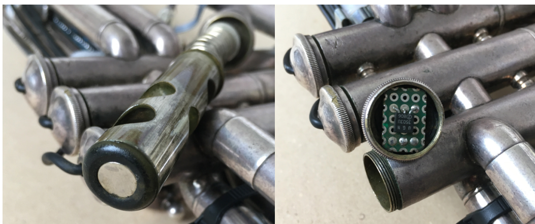
Figure 11: valves, showing magnet at base of piston (left) and Hall-effect sensor in base (right).
