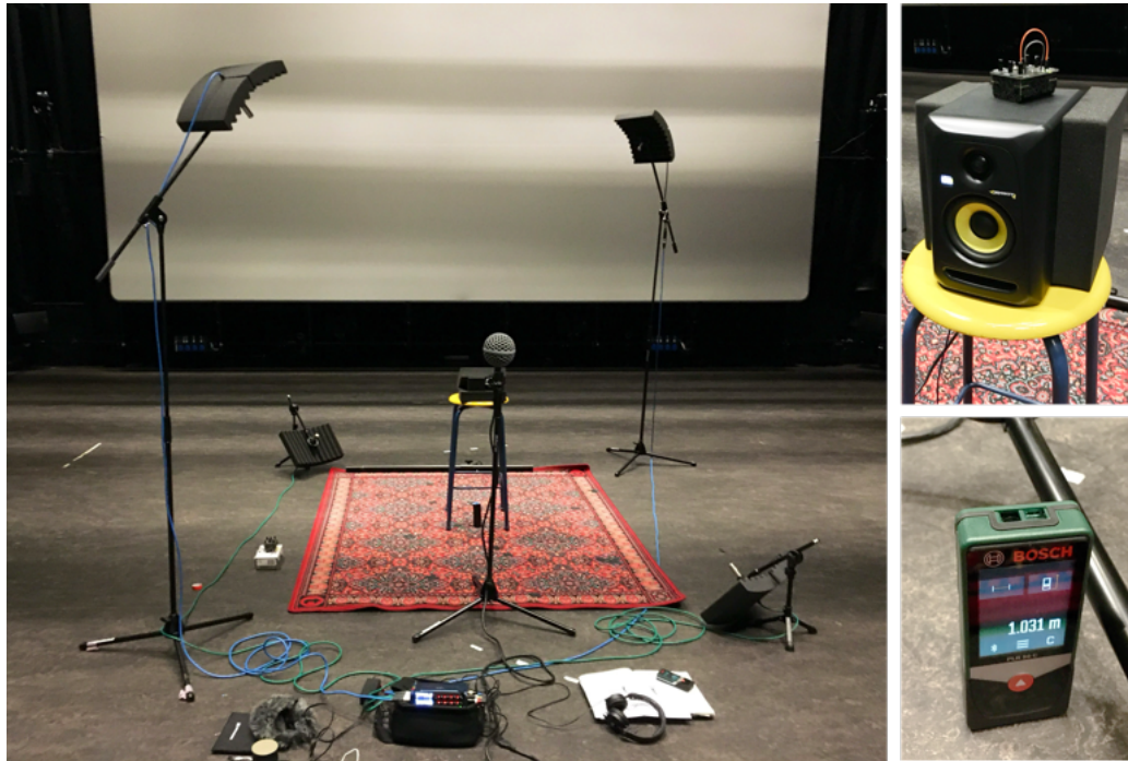
Figure 10. First test recording setup. CW from left: the sound object is temporarily replaced by an Ambisonics mic recording the "room tone": the sound object with distinct front/rear
